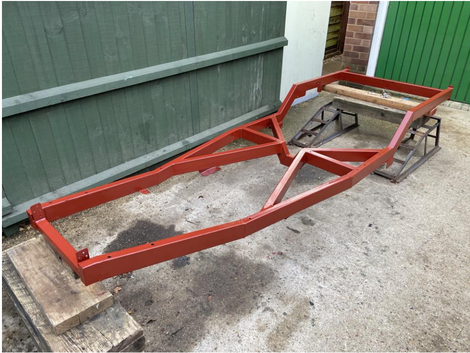
Note the absence of front engine mountings.
