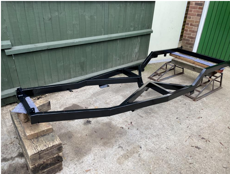
Finished in two coats of red oxide and two coats of agricultural gloss black.
